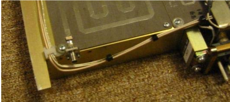
new RF connectors on input (left) and output (right)
